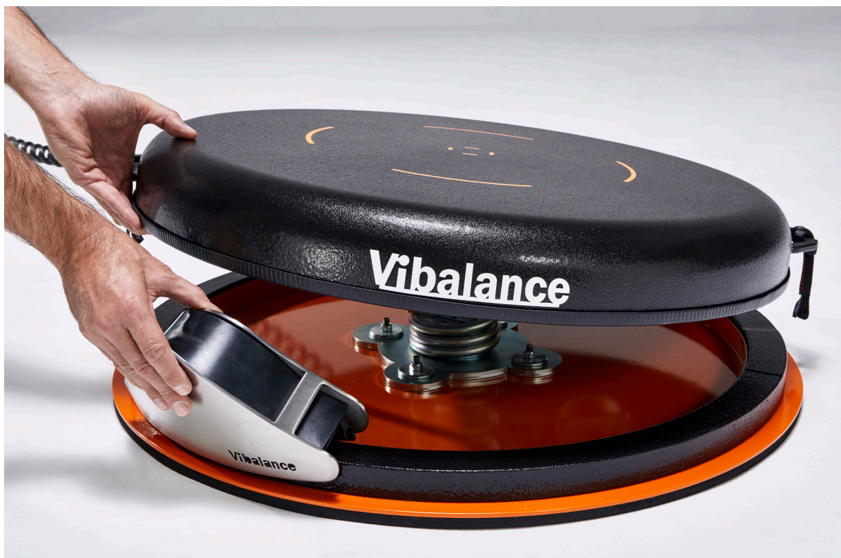
Figure 5a and 5b. Placing stabilizers on the base of the vibratory platform.
